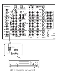
• The arrow on the cable connector body should be face down and lined up with the arrow below the connector on the amplifier for correct alignment. The i.LINK cable should be inserted straight into the connector so that it snaps easily into place. If not connected properly the amplifier will not be able to recognize any connected components. Note that the i.LINK cable is fragile and can be broken easily if too much force is used when connecting.
